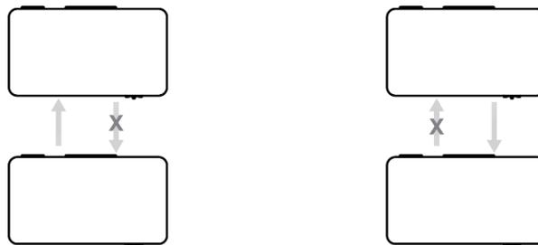
This is a conventional two way radio talk mode. It does not allow simultaneous 'transmit' & 'receive' functions.
