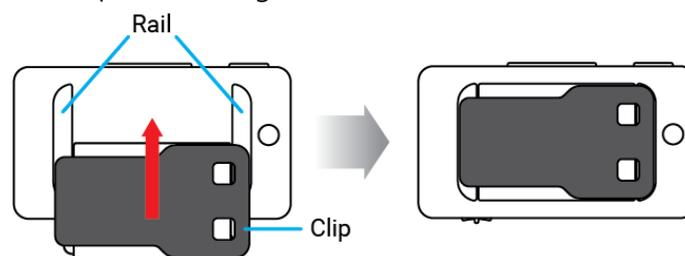
Slide the clip into the rail on the product and then push the clip upwards until you hear a 'click' as the arrow indicates.
