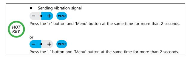
Your unit rings and vibrates and the vibration signal is sent.
