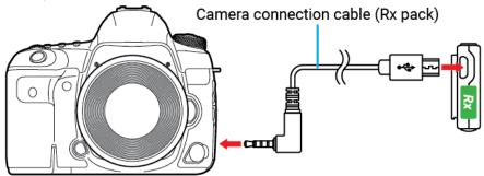
② Mobile devices such as smartphones, tablets and laptops need TRS to TRRS adapter included in the package between the device and the enclosed camera connection cable (Rx pack).
