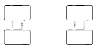
This is a conventional two way radio talk mode. It does not allow simultaneous 'transmit' & 'receive' functions.
