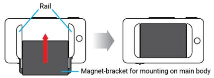
② The product with the magnet-bracket inserted can be attached on user's clothes together with the magnet-plate on the other side of user's clothes.
