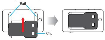
Slide the clip into the rail on the product and then push the clip upwards until you hear a 'click' as the arrow indicates.
